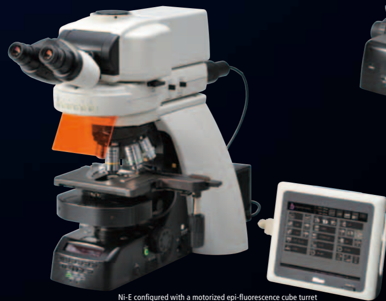
Ni-E configured with a motorized epi-fluorescence cube turret and motorized universal condenser
